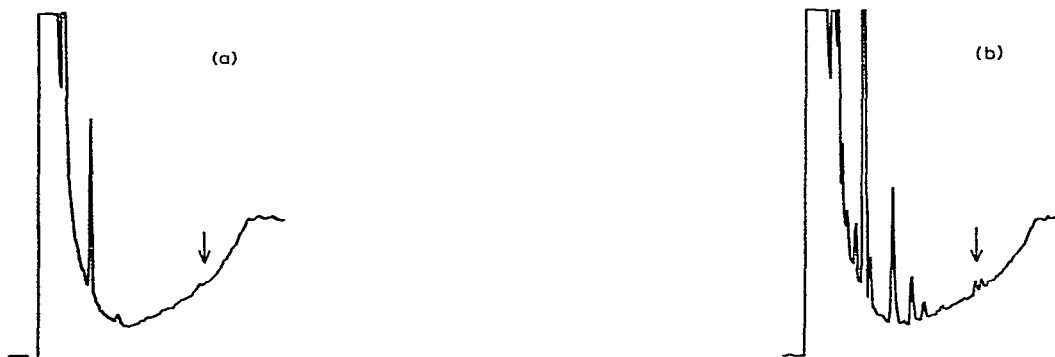
Fig. 5. Chromatogram of an acetone-1% 7-oxabicyclo(4.1.0)heptane solution. Volume injected: 5 \mu l. Flow-rate through column: ca. 30 ml/min ( N_2 ). Injector temperature, 220°C; detector temperature: 250°C. Temperature programme: 140°C (16 min), 2°C/min to 190°C (16 min). Detector: FID. Attenuation: 32. Recorder speed: 200 mm/h. (a) Before and (b) after ten-fold enrichment. The position of 2-chlorocyclohexanol is marked with an arrow.
